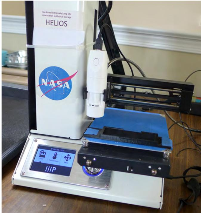
**Figure 8.** CTech designed and fabricated semi-automated spectroscopic reader for HELIOS media built on a modified 3D printer.
