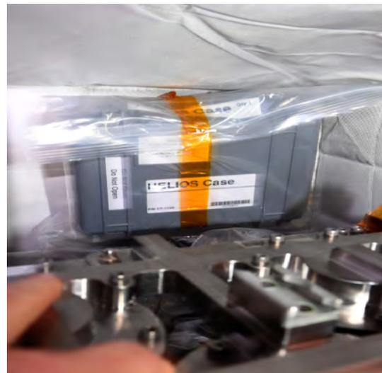
Figure 3. Sealed HELIOS case mounted in the ISS for maximum space radiation exposure.
