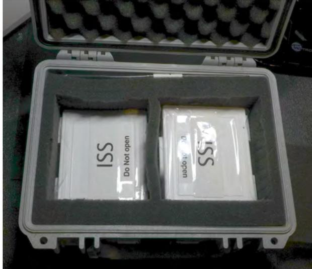
Figure 2. Opened ISS case showing two cassettes holding HELIOS test media.
