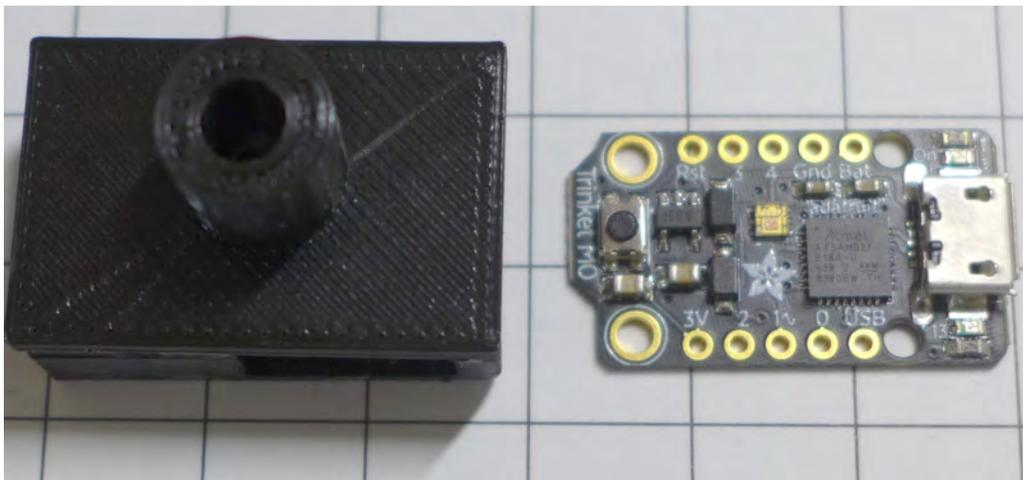
Figure 11. Adafruit Dotstar Trinket programmable light source for spectroscopic measurement of HELIOS media
