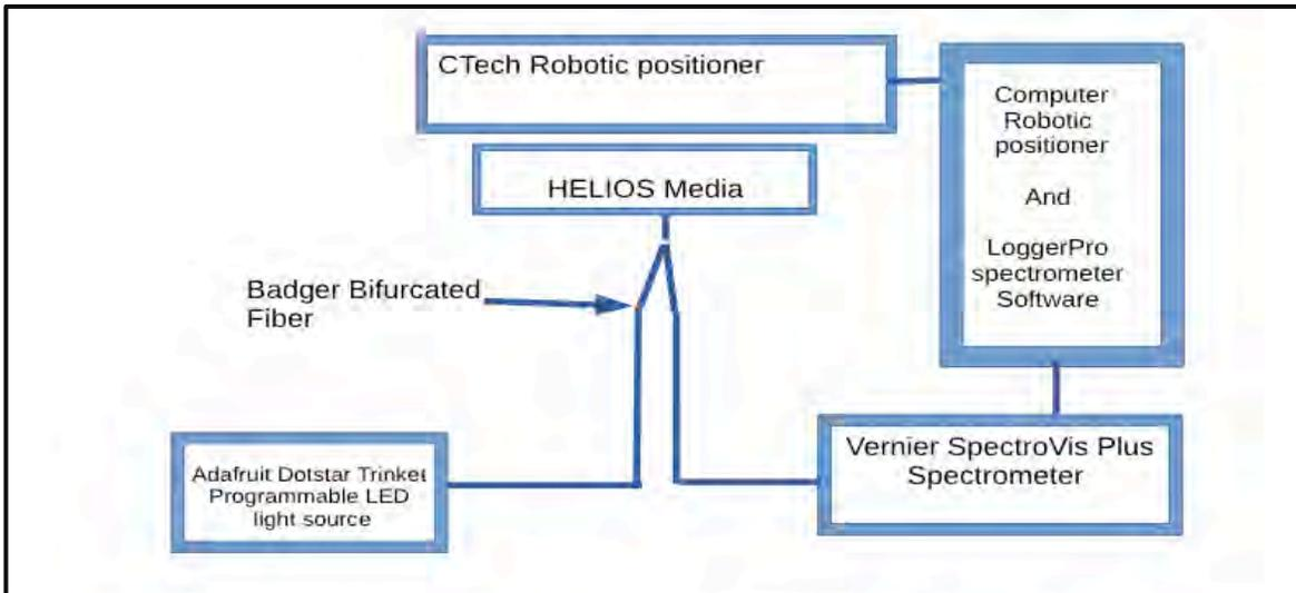
**Figure 13. Functional test setup for spectroscopic measurement of HELIOS media. (CTech, April 2020.)**
