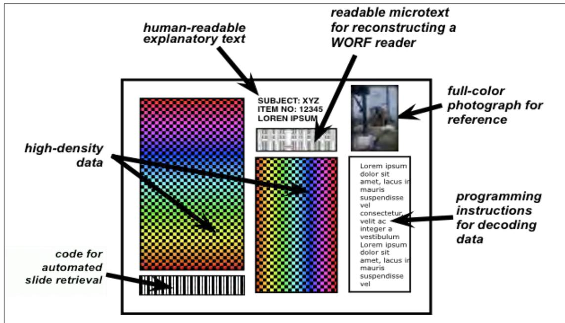
Figure 21. Example WOLF media layout showing various elements that can co-exist. Note that the size and shape of the media is agnostic — most any shape or size is feasible.
